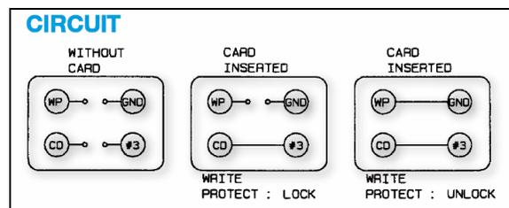
These extra signals are available on the SD connector, but not part of the SD specification, thus they aren't in any specific location manufacturer to manufacturer. Therefore, when designing SD card PCBs you will find that if you change the SD card connector, you will have to redesign the PCB footprint quite a bit.
