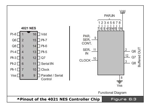
The NES controller is based on a parallel to serial shift register internally that "latches" the button states and then shifts them out to the host. The shift register used in the original NES control is the *CMOS 4021 shift register*. Figure 6:3 shows the pinout of the 4021 and the complete data sheet is on the CD located at:
