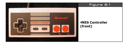
The classic NES controller / gamepad is shown in Figure 6:1, and internal shot is shown in Figure 6:2. As you can see there isn't much to the NES controller electronics (a single 4021 serial chip), but that's the beauty of it. The interface is so simple, we can use 4 lines to interface to the NES controller and read all 8 inputs (Up, Down, Left, Right, A, B, Select, Start).
