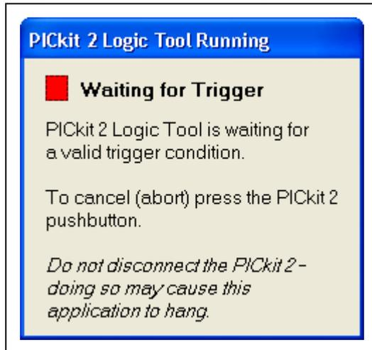
Once the trigger condition is met the “Busy” LED will turn off, the “Waiting for Trigger” dialog will close, and the analyzer waveform display will be updated with the newly captured data.
