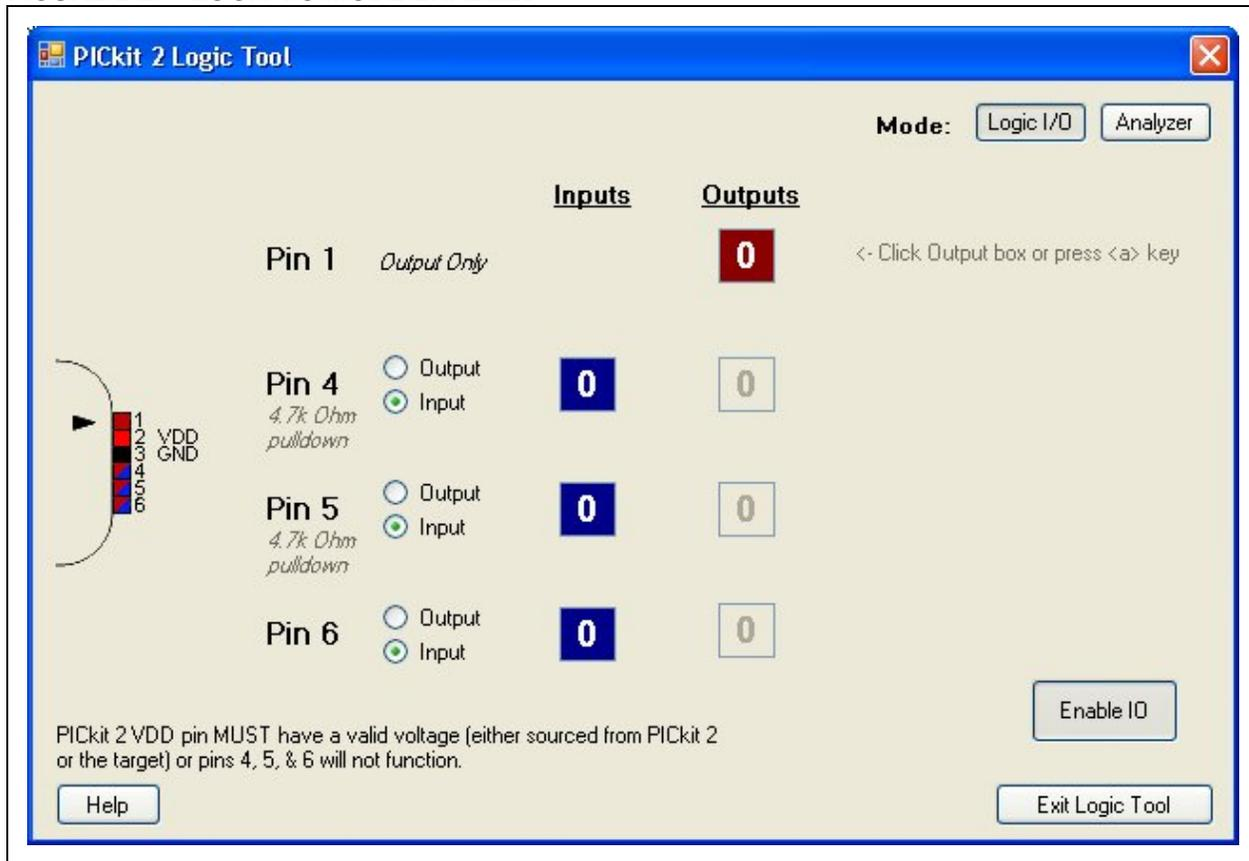
Now that the pins of the PICkit 2 unit are enabled, the pin directions and output states can be configured.
