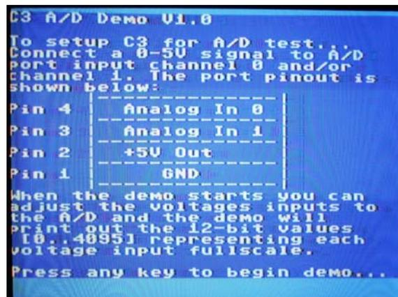
Figure 3.10 shows a screen shot of the demo running. I tried to use a little ASCII art to represent the actual signal header on the C3, so there is no confusion about what goes where. As you can see, you need to inject the signal(s) into pin(s) 3, 4, both or one. If you leave one open, I suggest grounding it so
