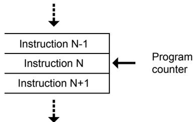
In Stage 1, instruction N, pointed to by the Program Counter, is fetched from cog memory during clock cycle M. During cycle M+1 the result from the previous instruction is written to memory. The reason the previous instruction result is written after the current instruction is fetched will be explained shortly.
