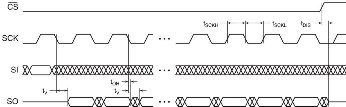
Figure 13-3.  $\overline{HOLD}$  Timing – Serial Input
