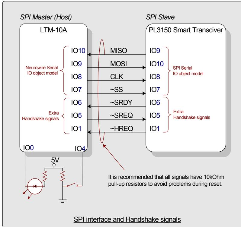
Figure 10. LMT-10A and PL 3150 Smart Transceiver Connections
