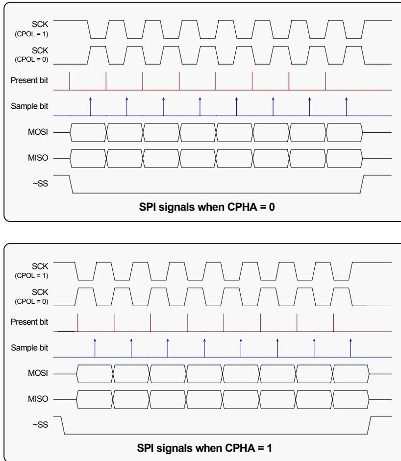
Figure 3. Clock Polarity and Clock Phase Settings
