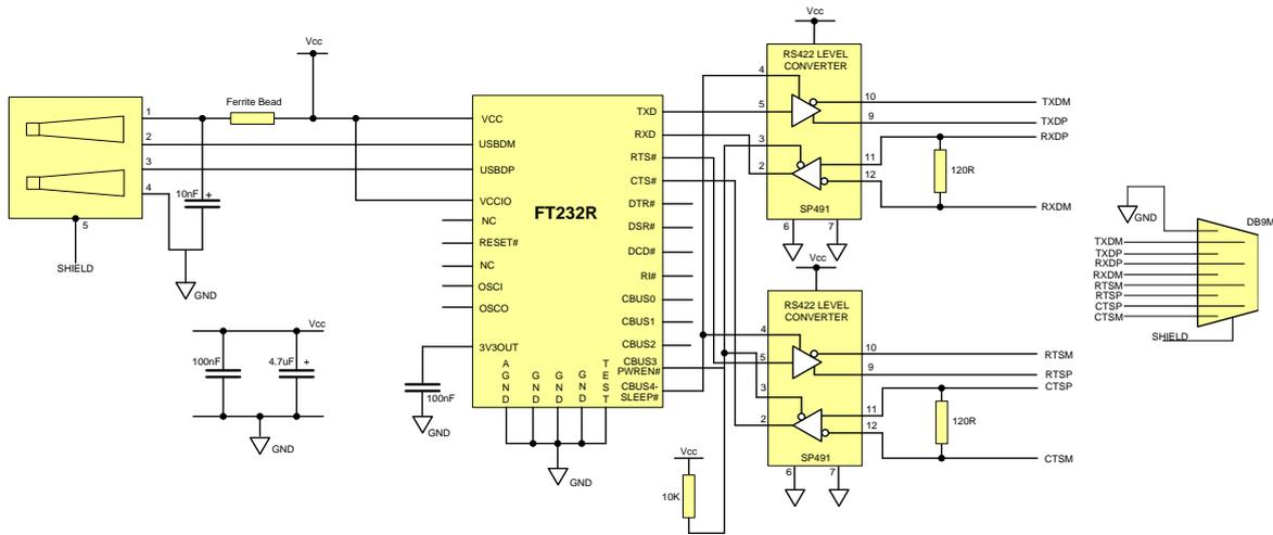
**Figure 7.3 USB to RS422 Converter Configuration**
