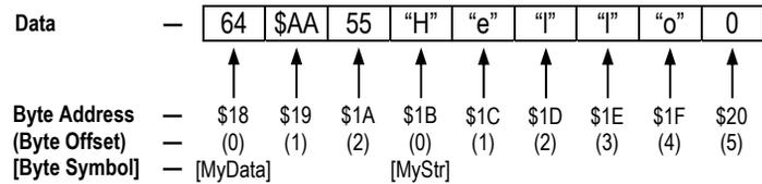
**Figure 2-1: Main Memory Byte-Sized Data Structure and Addressing**
