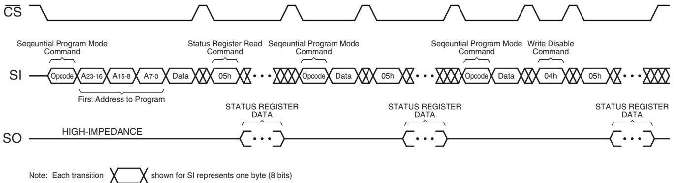
**Figure 8-4.** Sequential Program Mode – Waiting Maximum Byte Program Time
