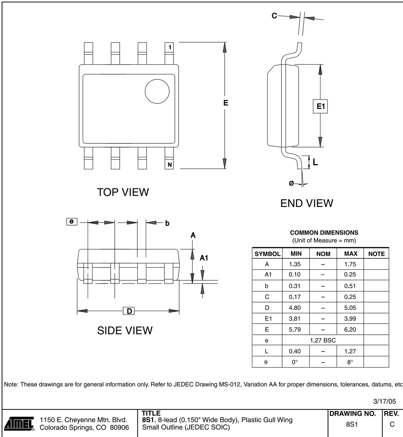
Note: These drawings are for general information only. Refer to JEDEC Drawing MS-012, Variation AA for proper dimensions, tolerances, datums, etc.
