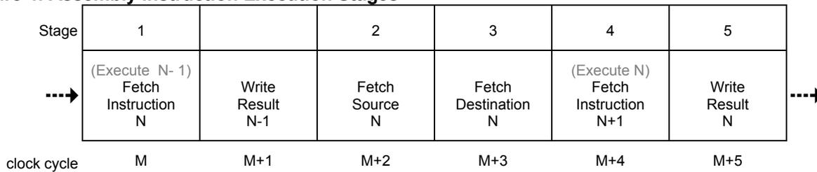
The Propeller executes assembly instructions in five stages. While an entire instruction takes six cycles to execute, two of those clock cycles are dedicated to the two adjacent instructions. This results in an overall throughput of four clock cycles per instruction.
