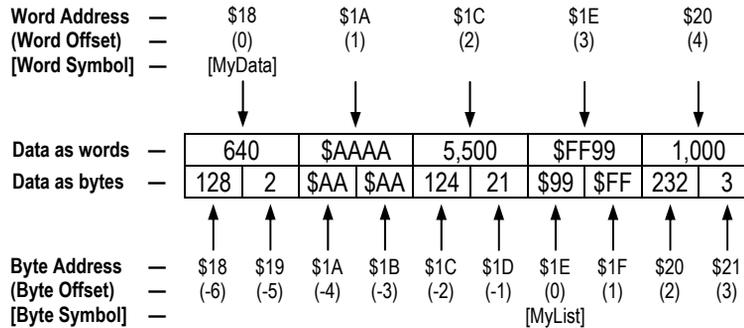
**Figure 2-5: Main Memory Word-Sized Data Structure and Addressing**
