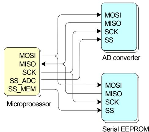
Figure 1. One Master and Two Slave Peripherals
