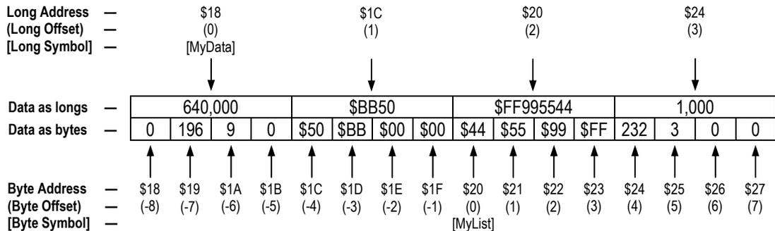
**Figure 2-2: Main Memory Long-Sized Data Structure and Addressing**
