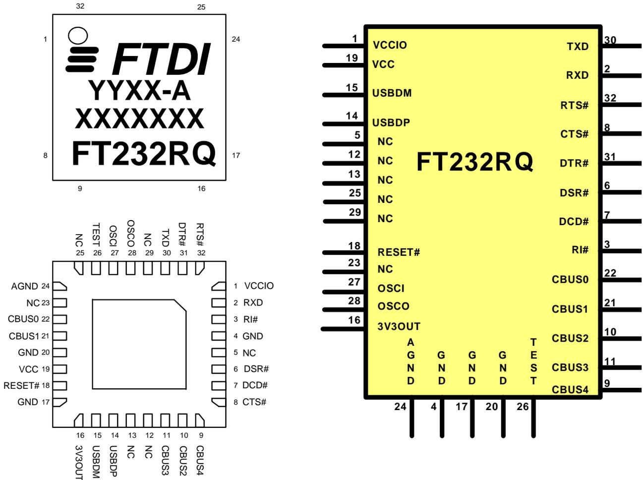
Figure 3.2 QFN-32 Package Pin Out and schematic symbol
