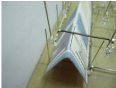
(b) The triangle supports provide separation distance about 2.5cm height
