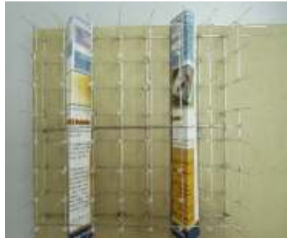
(b) Move around the triangle support during the soldering process
