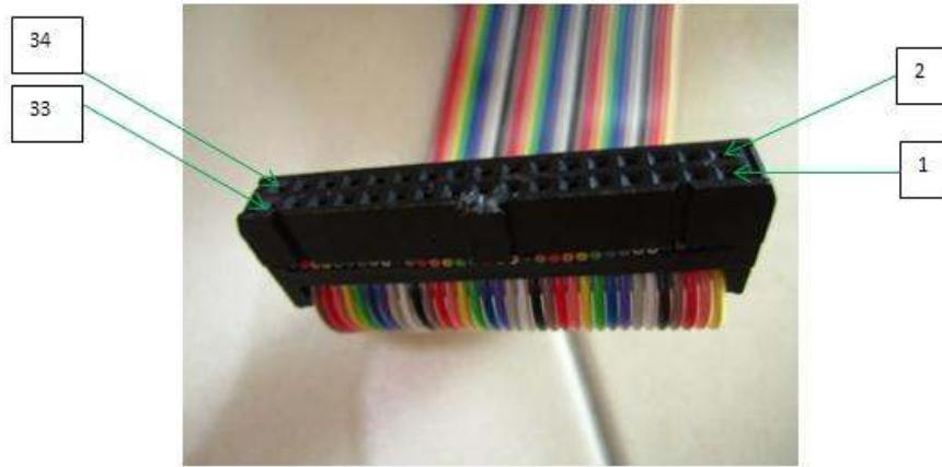
Figure 62: Wires connection to IDC socket slots
