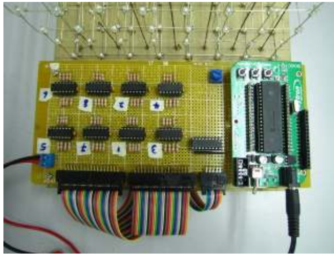
Figure 88: Attach the microcontroller circuit board to the base of the LED Cube
