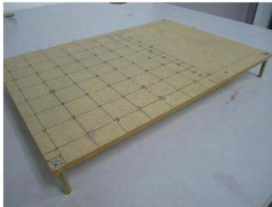
Figure 39: Stack up the base using PCB stands
