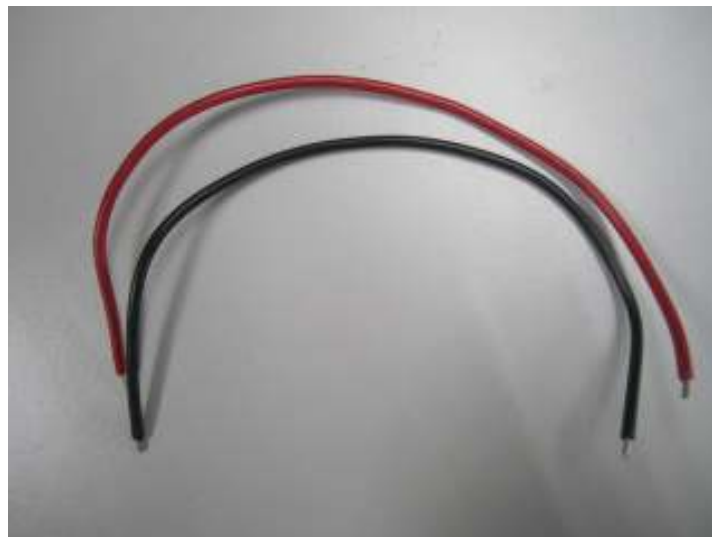
Figure 83: 2 cut out Multicore wire AWG 14 (WR-MM14) (1 Black and 1 Red) for 5V supply from BB-ATXRA to microcontroller board
