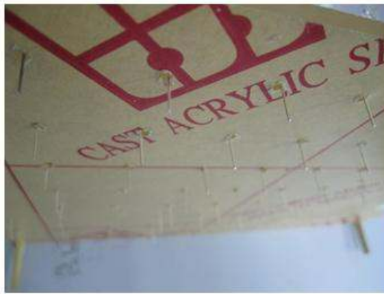
a) Cut the anode legs into length about 1cm long
