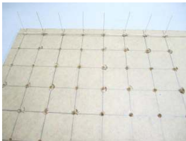
(c) Row of LEDs with their cathodes connected together by soldering the cathode and cathode contact points
