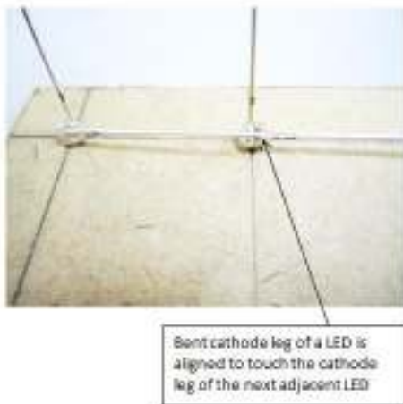
(a) Contact between cathode of a LED with the next adjacent LED
