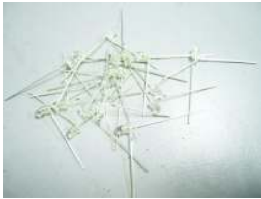
Figure 13: Bend up LEDs cathode leds 90 degree up
