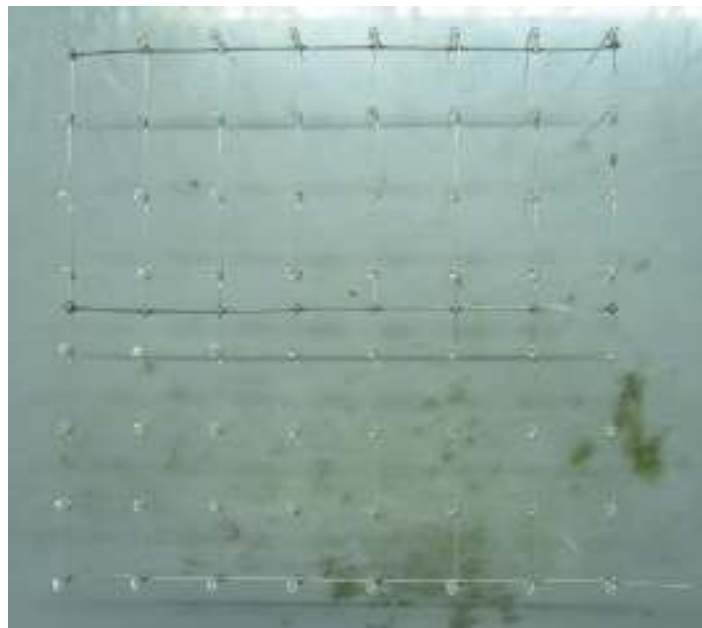
Figure 22: The appearance of the LEDs layer taken out from the mold
