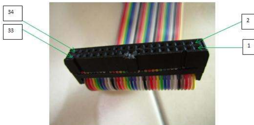
Figure 64: Wires connection to IDC socket slots
