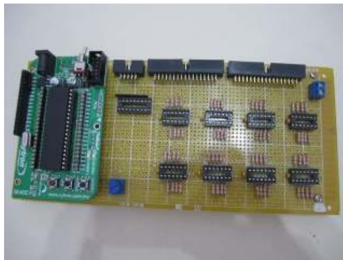
Figure 76: Appearance of the microcontroller circuit board when SK40C is plugged in to the assigned headers
