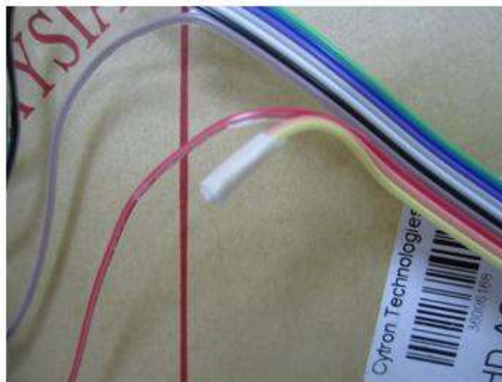
Figure 49: Cut off extra part of the unused wires
