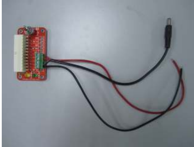
Figure 84: The resulted connections of wires to BB-ATXRA
