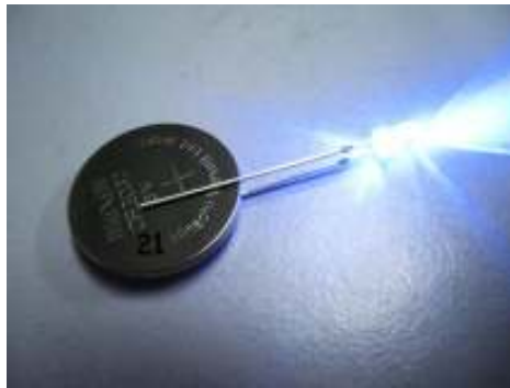
Figure 12: Checking a LED functionality using 3v Cell Battery CR2032
