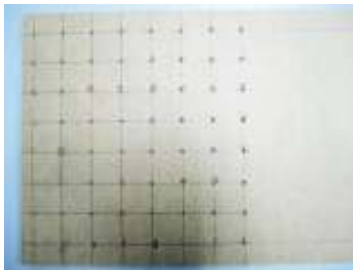
Figure 3: Mold to facilitate soldering process of LEDs
