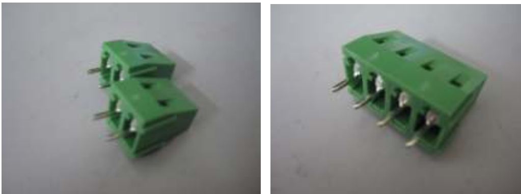
Figure 80: A 4 ways terminal block resulted from two ways terminal block
