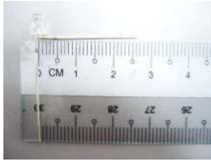
Figure 8: Super bright 3mm blue LED with its cathode leg bent 90 degree
