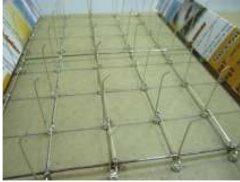
(b) Bend small section of all anode legs of LEDs in the lower LEDs layer
