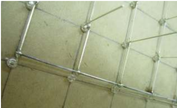
c) Solder all contact points between cathode legs and the brace
