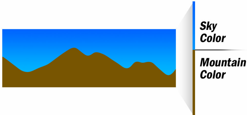
Figure 9.2 – Analyzing 1-pixel vertical strips of the mountain range graphic.
