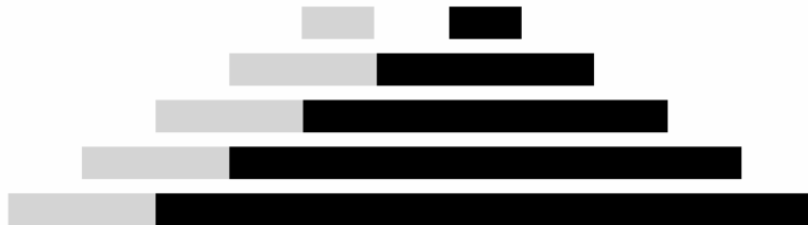
Figure 9.5 – Shifting the track left or right by adding an unchanging value to each scanline's data points.
