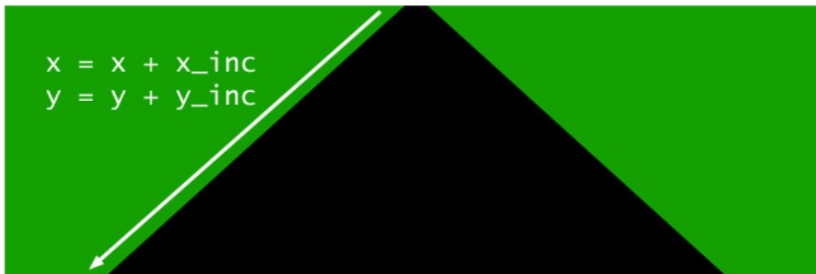
Figure 9.4 – Using tracking variables to follow the slope of a line as the track is drawn down the screen.
