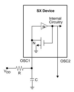
Figure 4-1 External RC Oscillator Connections
