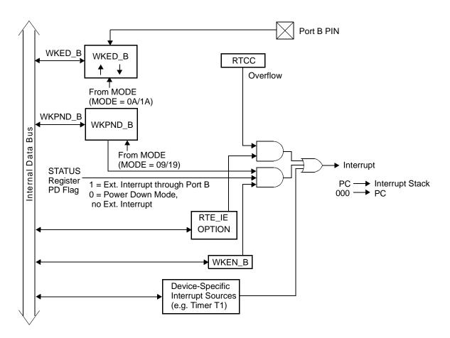
Figure 6-2 Interrupt Logic Block Diagram
