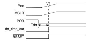
Figure 4-7 Power-On Reset Timing, V<sub>DD</sub> Rise Time Too Slow
