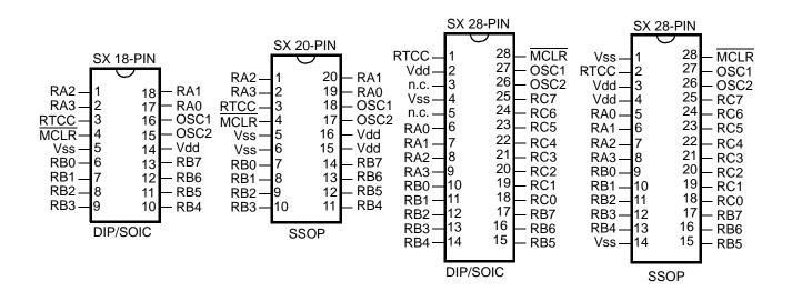
Figure 1-1 SX18/20/28 Pin Assignments
