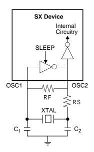
Figure 4-2 Crystal or Ceramic Resonator Connections
