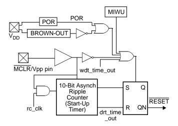
Figure 4-5 On-Chip Reset Circuit Block Diagram
