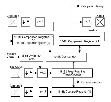
Figure 8-1 Multi-Function Timer Block Diagram
