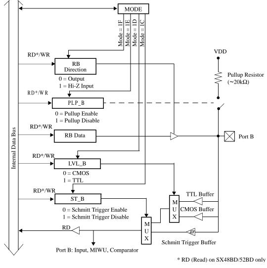
Figure 5-1 Port B Pin Block Diagram
