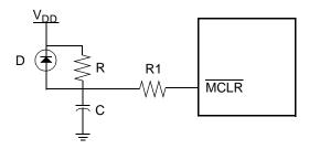
Figure 4-8 External Power-On MCLR Signal
