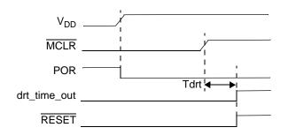
Figure 4-9 Power-On Reset Timing, Separate MCLR Signal
