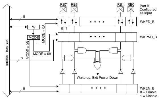
Figure 4-4 Multi-Input Wakeup/Interrupt Block Diagram
