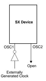
Figure 4-3 External Clock Signal Connection
