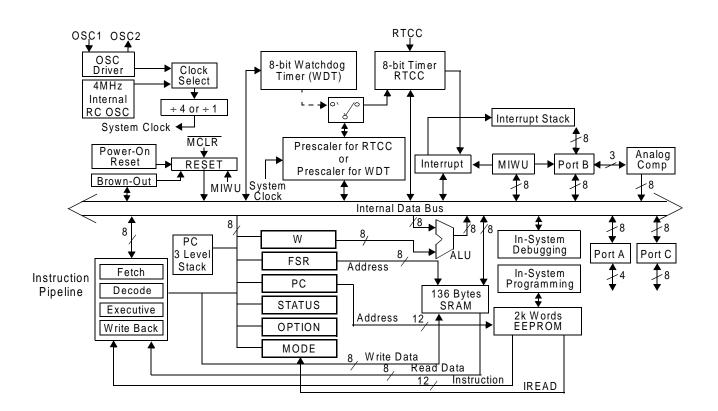
Figure 2-1 SX28AC Block Diagram
