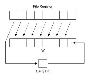
Figure 3-2 Rotate fr Left Through Carry into W
