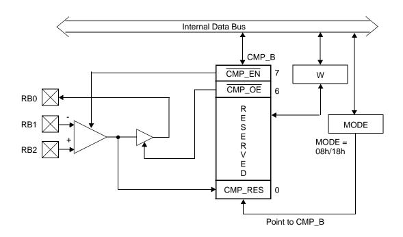
Figure 7-1 Comparator Block Diagram
